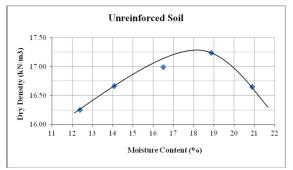
Figure.3 Maximum Dry Density for Unreinforced Soil
