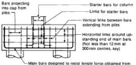
table below (A, = tension/0.87f,). Ends bent and carried to top of cap as shown. Not less than 0.25% of mild steel or 0.15% of high-yield steel
