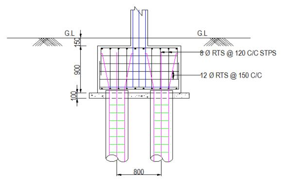
REINFORCEMENT DETAILS OF TWO PILE GROUP
