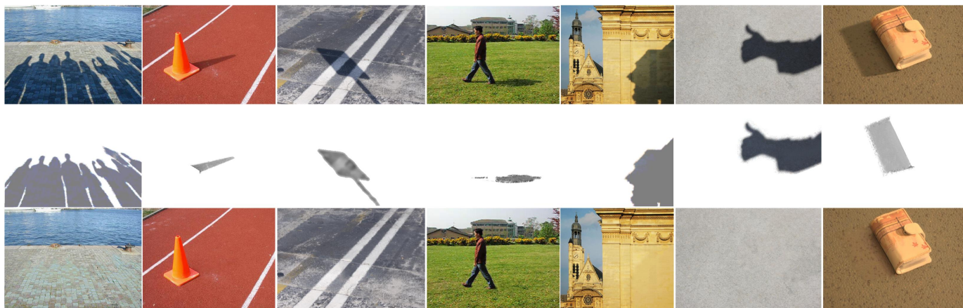
Fig. 12: Qualitative Evaluation: Shadow recovery on sample images from UIUC, UCF databases and other images used in literature. Given a original image with shadow mask ( first row ), our method is able to extract exact shadows ( second row ) and to automatically recover the shadow-less images ( third row ). ( Best viewed in color )
