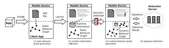
Fig. 2. Overview of MONET. Runtime behavior signature will be generated through static behavior graph generation, runtime information collection and runtime behavior graph generation.
