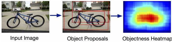
Fig. 3. An illustration of objectness generation process for assessing the easiness of an image sample.
