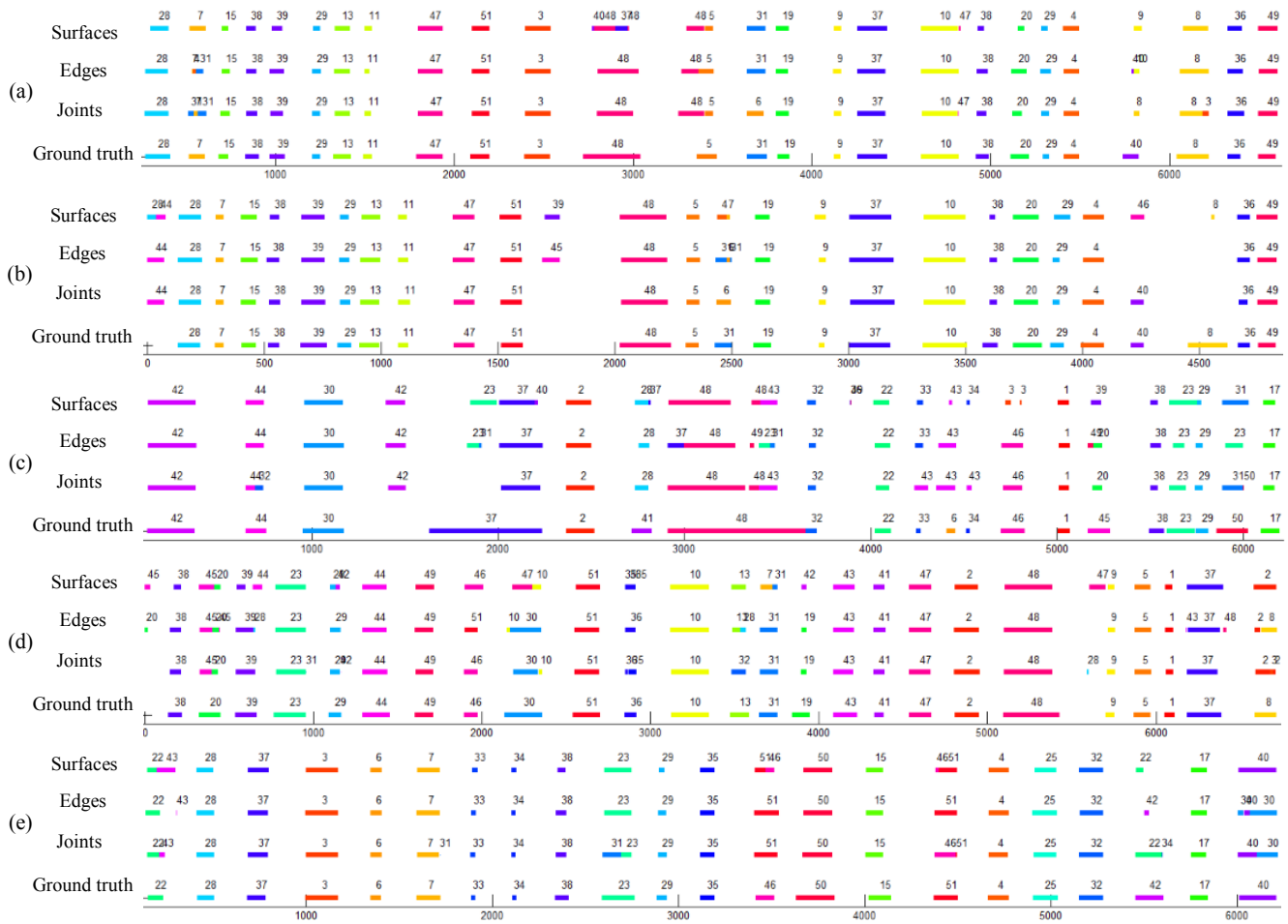
Fig. 6. Visualizations of action detection. Here, we show results of five samples on the validation set of the PKU-MMD dataset. The x-axis represents the frame index, and each line segment along the time axis denotes an action interval. The number above the segment denotes the action class index.
